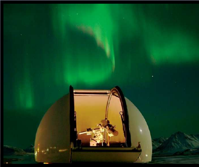
Starphotometer STAR01 (S & P) and 3.2 m Baader observation dome at Koldewey-Station on Spitsbergen (Norway)
