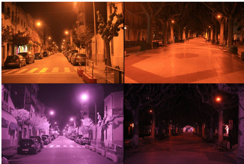
Figure 6: Street scenes in Tremp. Top: visual light, left: sodium high pressure, illumination levels 50-60 lx, right: pc amber LED, illumination level 35 lx. Bottom: near infrared light, filtered with a 730 nm filter: sodium has bright emission lines at 818/819 nm.
